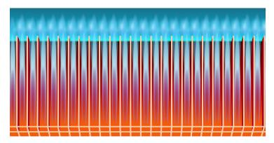
By adding a ducted ceramic tile above a standard burner, Duplex essentially turns a single large and unruly flame into thousands of tiny, more easily controlled flames. Duplex burner architecture reduces flame length by more than 80%
